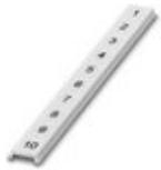
Zack Marker strip, flat, Strip, white, labeled, Printed vertically: consecutive numbers 1 ... 10, 11 ... 20, etc. up to 91 ... 100, mounting type: snap into flat marker groove, for terminal block width: 6.2 mm, lettering field size: 5.15 x 6.15 mm, Number of individual labels: 10
