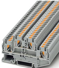
Double-level terminal block, nom. voltage: 500 V, nominal current: 28 A, connection method: Push-in connection, 1st and 2nd level, Rated cross section: 4 mm<sup>2</sup>, cross section: 0.2 mm<sup>2</sup> - 6 mm<sup>2</sup>, mounting type: NS 35/7,5, NS 35/15, color: gray
