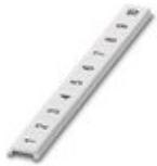
Zack Marker strip, flat, Strip, white, labeled, printed horizontally: consecutive numbers 1 ... 10, 11 ... 20, etc. up to 91 ... 100, mounting type: snap into flat marker groove, for terminal block width: 6.2 mm, lettering field size: 5.15 x 6.15 mm, Number of individual labels: 10
